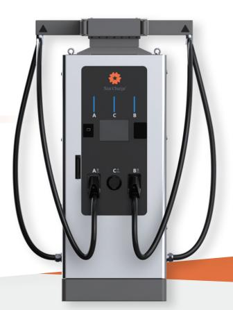
**Jupiter** provides a versatile 3-in-1 charging solution with an impressive 95% efficiency. It offers flexible configuration options, including two rapid DC charging connectors with a maximum output of 60 kW for scenarios where quicker recharges are preferred, as well as an 22 kW AC socket for slow charging mode. Designed to accommodate various needs in destination charging environments, Jupiter is compatible with 99% of electric vehicles, ensuring broad market applicability.
